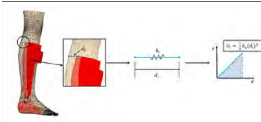
Figure 1: Linear spring model of AFO and leg.
