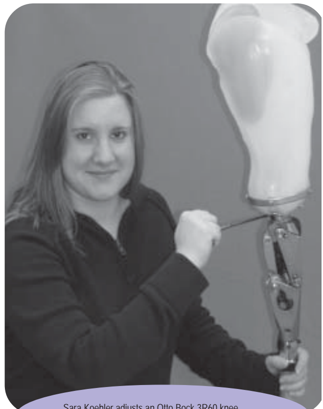
Sara Koehler adjusts an Otto Bock 3R60 knee designed to manage impact forces during gait.
