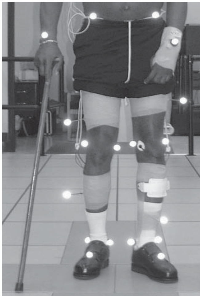
Figure 3: The Helen Hayes marker set used during the gait analysis. Reflective markers were taped to the skin over both Anterior Superior Iliac Spines (ASIS), femoral condyles, malleoli, dorsum (top) of the feet, laterally on the thighs and shanks (wand markers), and the sacrum and heel (not shown in photo). Data from markers placed on the trunk and upper limbs were not used in this study. Where the AFO obscured the landmarks required for identification of the ankle joint axis, markers were screwed into the mechanical ankle joint. Medial markers are used in the calculation of joint centers of rotation and were removed after collection of a single static trial. Surface electrodes, with the exception of the ground electrode on the tibial plateau, were taped down and the leads were connected to a telemetry pack worn on a backpack-style harness.
